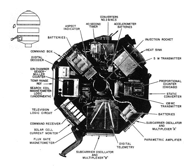
Figure 8. Able-3 Payload (Top View).
