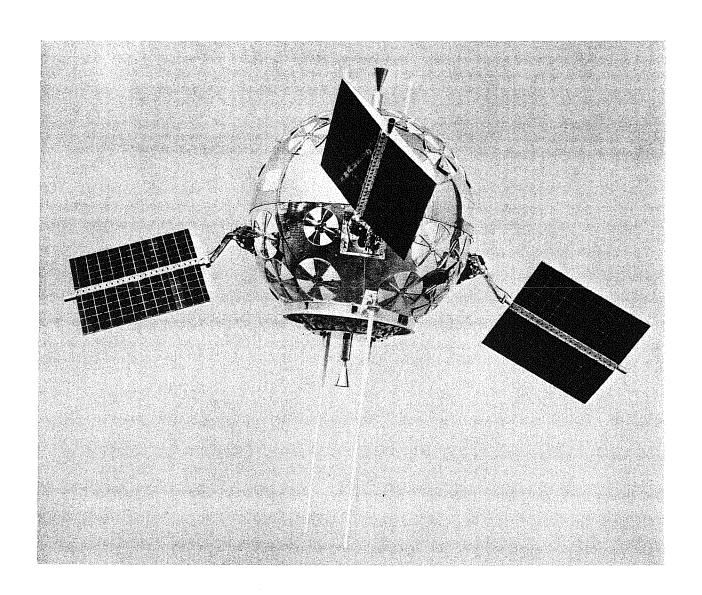
Figure 15. The Able-4 Atlas Payload.
