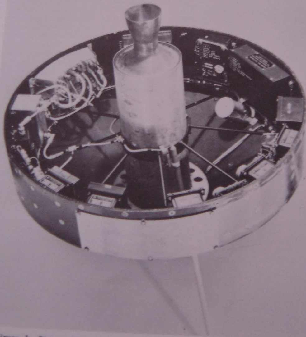
Figure 1. Pioneer II payload. Oblique view showing micrometeorite diaphragm and one leg of the dipole antenna
