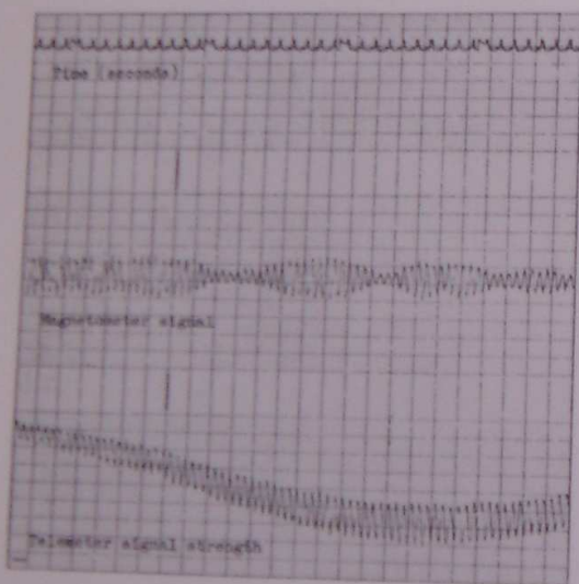
Figure 8. Magnetometer signal showing almost periodic variations in the value of H
